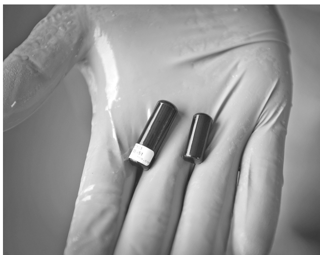
A close-up view of transmitters used to track fish is shown. (courtesy of DNR)
